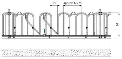
Sectional view installed feed front 140<sup>+</sup>-145<sup>+</sup>
