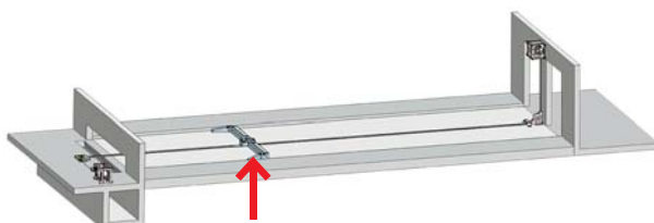
▲ 28/2 Scraper is standing in the walkway (wrong)
